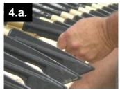
Loosen the receptor's lock nut from the carriage bolt and adjust the angle of the nylon finger.
