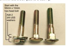
NOTE: Using the above configurations, the hexhead bolt may wear over time, in which case it will be difficult to remove without cutting or grinding it off. The hex-head may also catch plant material and rocks under the header.
