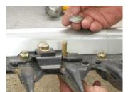
Place washers of the appropriate size and numbers onto the protruding bolt.
