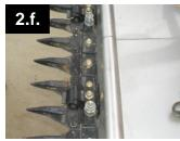
f. Install the remaining QD<sup>TM</sup> nuts on the rest of the header using the first-installed QD<sup>TM</sup> nut as a guide. When necessary to install a QD<sup>TM</sup> nut assembly on a knife hold down, the number of washers required will need to be reduced by the thickness of the knife hold down.
